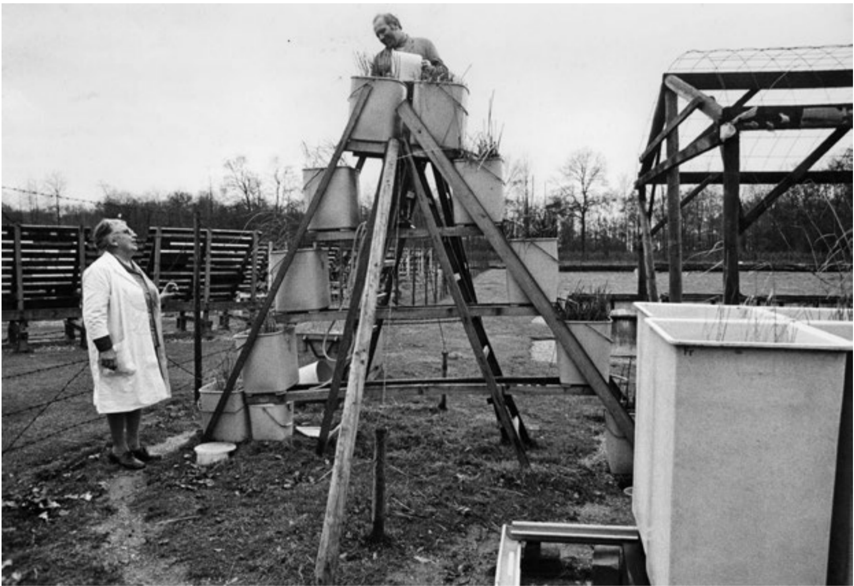
The Krefeld System, an experimental set-up involving roof battens, wire mesh and plastic buckets designed to clean wastewater
